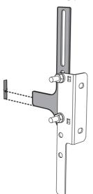
3. Align the base of the fastening bracket with the ground and tighten the screws to fix the measurements.
