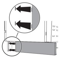
4. Line up the hole on the side skirting with the rear hole on the base of the appliance.
