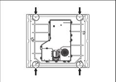
Fasten the fixing brackets (A) into the holes marked using the screws that were removed in order to correctly fix the hob to the structure.
