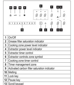
The cooking zones can be activated by pressing the reference digit  $\Box$ . The digit becomes brighter to confirm the operation.
