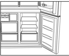
1- Sealing is provided when the gaskets on the door presses on the surface of the movable middle section while the fridge compartment doors are closed.
