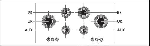
AUX: Auxiliary burner SR: Semi-rapid burner R: Rapid burner
