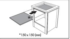
\*necessary for gas connection With opening on bottom or back:
