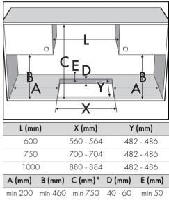
\* If there is a kitchen unit positioned above the hob. In the case of a hood, refer to the measurements indicated in the relative manual.
