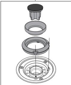
Before lighting the hob burners, make sure that the flame-spreader crowns are correctly positioned in their housings with their respective burner caps. Make sure that the holes in the burners are aligned with the thermocouples and the spark ignitions. Also ensure that the flamespreader crowns are correctly engaged in the burner holes.
