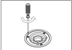
Remove the screws that fasten the hob top to the burner casing (the figure shows the 60 cm model as an example Burner) for each burner.
