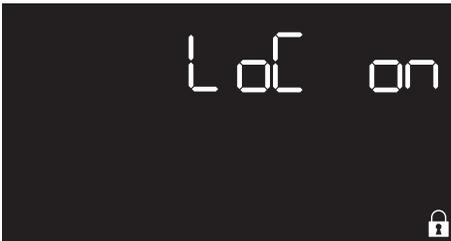
**i** During normal operation, the controls lock is indicated by the
