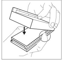
4. Remove the top glass shelf from the fridge compartment. Slip the plastic housing with the air filter on the left side of the glass shelf.
