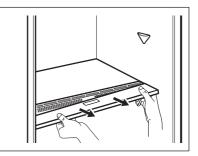
(1) Depending on the quantity and condition of fruit and vegetables stored in the GreenZone drawer, condensation may occur. In such a case, remove the condensation using a soft cloth and set the humidity control to low humidity position.
