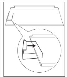
5. Insert the glass shelf back in the fridge compartment. Be careful not to hit the filter when inserting the glass shelf.
