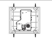
Fasten the fixing brackets (A) into the holes marked using the screws that were removed in order to correctly fix the hob to the structure.
