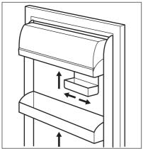
This model is equipped with a variable storage box which can be moved sideways.
