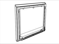
4. Place the internal glass panel back onto the brackets after cleaning. Make sure that you centre and then insert the 4 pins firmly into their housings on the door with the help of the strips at the right and left in order to achieve a perfect fit.
