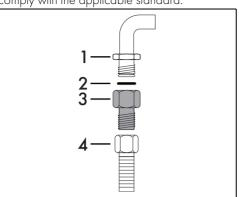
Carefully screw the hose connector 3 to the appliance's gas connector 1 (1/2" thread ISO 228-1), placing the seal 2, provided, between them. Apply insulating material to the thread of connector 3 and then screw the steel hose 4 onto the connector 3.
