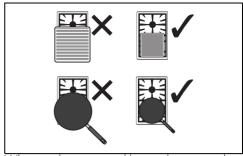
When cooking, to avoid burns, damage to the hob or top, all containers or steak pans must be positioned within the perimeter of the hob.
