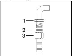
Carefully screw the connector 3 to the gas connector 1 of the appliance, placing the seal 2 between them.
