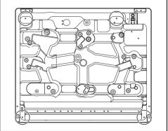
Screw the fixing brackets into the dedicated holes as shown to properly fasten the hob to the
