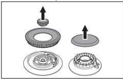
4. Remove the gasket on each burner's thermocouple and igniter.
