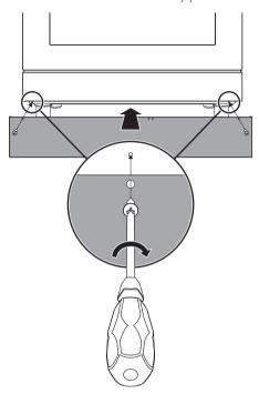
3. Fasten the front plinth to the appliance using the screws that were previously removed.
