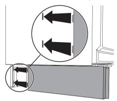
4. Line up the holes of the side plinth with the hole at the rear of base of the appliance.
