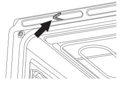
During normal cleaning operations, the door lock lever may be activated accidentally.
