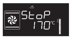
6. To turn off the buzzer, press or turn one of the two knobs or open the door.
