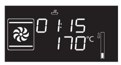
A few seconds after having set the required duration, the indicator light stops flashing and timed cooking starts.
