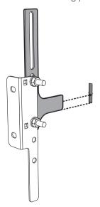
5. Align the base of the fastening bracket so that it reaches the floor and tighten the screws to fix it in position.
