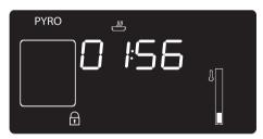
1. The display indicates and the remaining time to indicate that the appliance is carrying out the automatic cleaning cycle.
