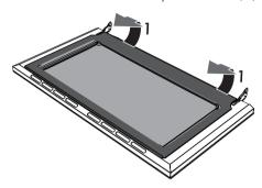
2. Remove the internal glass panel from the front strip (2) to remove it from the door
