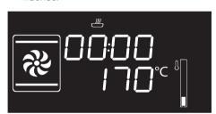
2. Turn the temperature knob to the right or left to set the cooking duration from 00:01 to 12:59. Keep the knob turned to produce a faster increase or decrease.
