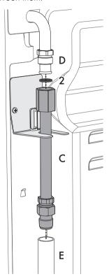
5. Apply insulating material to the thread of the extension pipe assembly C, then tighten the hose E.
