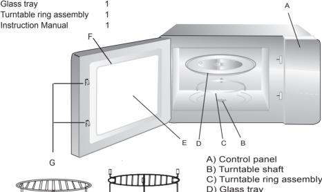
Grill Rack( Only be used in grill function and be placed on the glass tray)
