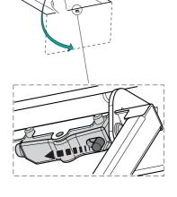
• Screw the Frame into place using the 6 screws **12f**, reconnect the wires to the Commands and Light, replace the metal grease filter and the Panel.
