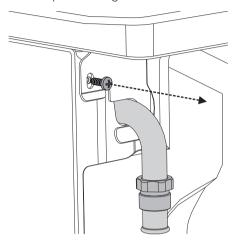
2. Attach the chain to the cooker with the screw just removed.
