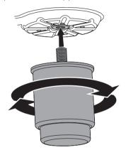
The appliance must sit level on the floor to ensure stability.
