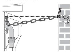
5. Drill the hole and insert a wall plug.
