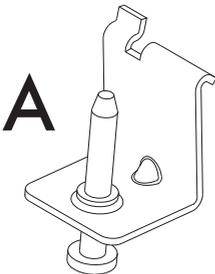
3. Place the hob on the insulating seal and fix it to the supporting structure using the supplied screws and fastening brackets (A) so that the hob is perfectly level.
