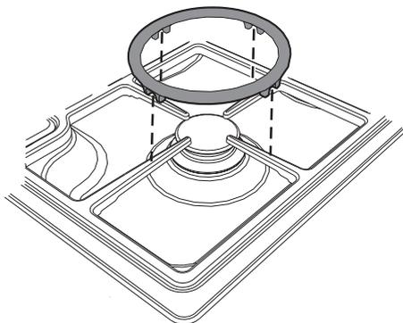
The ring must be placed under the hob grid as shown in the picture above.
