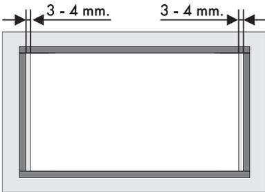
2. Make the seal stick to the edge around the hole cut in the worktop, using a slight pressure; front and rear sides of the seal must brush against the hole.
