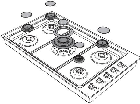
3. Replace the burner nozzles using a 7 mm socket wrench according to the gas to be used (see "Burner and nozzle characteristics tables").
