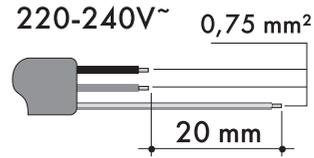
Use a **3 x 0.75 mm<sup>2</sup> three-core** cable.
