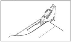
Grasp the door on both sides with both hands, lift it so that it forms an angle of around 30° and remove it.
