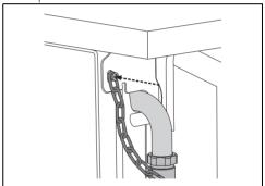
Stretch the chain out horizontally so that the other end touches the wall. Mark the position for the hole on the wall.
