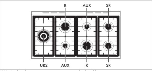
AUX = Auxiliary Burner SR = Semi-rapid Burner
