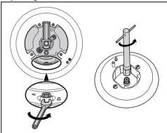
Remove the pan supports, burner caps and flame-spreader crowns to access the burner cups.
