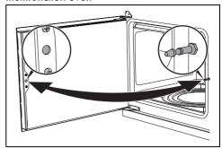
Multifunction ovens are equipped with a swing door. To open, pull the door handle towards you. To close, push the doors until you hear a mechanical "click".
