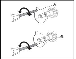
Light the burner and turn it to the minimum position. Extract the gas cock knob and turn the adjustment screw next to the gas cock spindle
