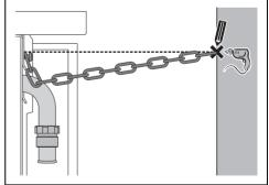
Drill a hole at the marked position and insert a wall plug.
