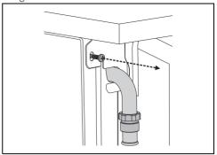
Attach the chain to the cooker using the screw that was removed in the previous step.
