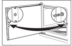
Multifunction ovens are equipped with a swing door. To open, pull the door handle towards you. To close, push the doors until you hear a mechanical "click".
