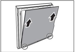
3. After removing the inner glass, it is possible to access the drip catcher strip.
