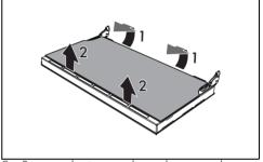
3. Remove the intermediate glass pane by lifting it upwards.
