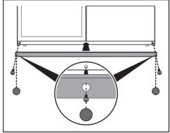
The plinth must always be positioned and secured correctly on the appliance.
