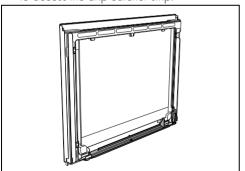
4. Place the internal glass panel back onto the brackets after cleaning. Make sure that you centre and then insert the 4 pins firmly into their housings on the door with the help of the strips at the right and left in order to achieve a perfect fit.
