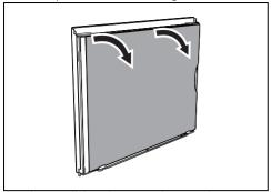
Then, pull the glass panel upwards, paying attention to the brackets at the bottom of the door.
