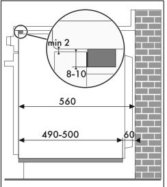
If the appliance is to be built-in under a worktop, a wooden bar has to be installed order to use the seal that is glued to the back of the front panel to prevent water or other liquids leaking in.
