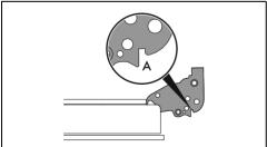
4. Lower the door and once it is in place remove the pins from the holes in the hinges.
