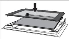
The intermediate glass pane must be repositioned on the open door so that the screen printing in the corner can be read from left to right (the rough part of the screen printing must face the external glass pane of the door).
