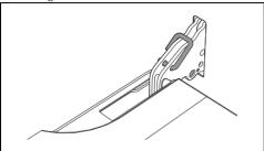
Grasp the door on both sides with both hands, lift it forming an angle of around 30° and remove it.
