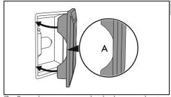
Press the cover completely down so that it attaches perfectly to the bulb support.
