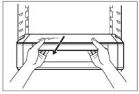
**2.** Tilt the module downwards to remove it from the refrigerator.
