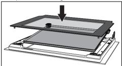
The intermediate glass pane must be repositioned on the open door so that the screen printing in the corner can be read from left to right (the rough part of the screen printing must face the external glass pane of the door).
