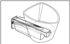
Pour the water (using a bottle or a measuring jug) until the max. level indicator light comes on (the reservoir contains about 800 ml of water).
