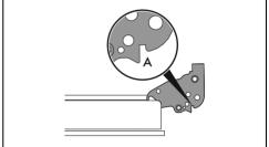
Lower the door and once it is in place remove the pins from the holes in the hinges.
