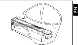
4. Pour the descaling solution into the funnel.
