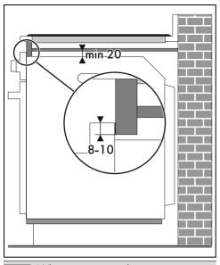
When using a wooden separator, a wooden bar has to be installed under the worktop in order to use the seal that is glued to the back of the front panel to prevent water or other liquids leaking in.
