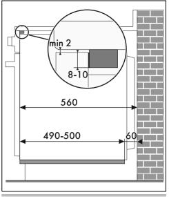
If the appliance is to be built-in under a worktop, a wooden bar has to be installed order to use the seal that is glued to the back of the front panel to prevent water or other liquids leaking in.
