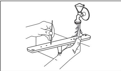
3. To install the spray arm back, press it downwards.
