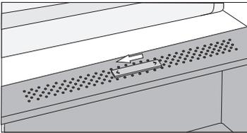
**Slider position to the left:** open vents, lower humidity in the bin
