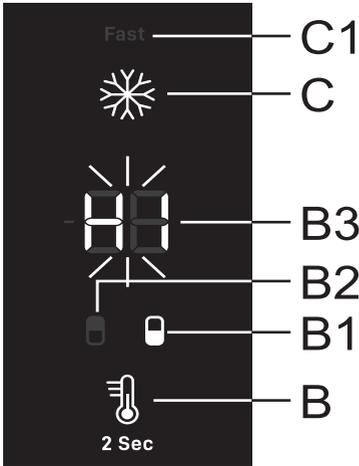
If the temperature inside the appliance is too high, then an acoustic alarm will be activated (**intermittent tone**). HI will flash on the **B3** display unit, and the symbol for the part of the appliance where the temperature is too high (**B1** or **B2**) will be lit.
