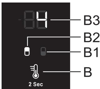
In this model, you can switch between setting the temperature of the refrigerator and the temperature of the freezer compartment. To do this, press the **B** key and hold it for two seconds until the symbol for the desired compartment lights up: **B1** for the freezer compartment and **B2** for the refrigerator compartment.
