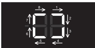
**Switching off the appliance:** To switch off the appliance, press the **A** key and hold it for a while (2 seconds). A beep will be sounded again and the outer segments of the display digits **B3** will light up in the clockwise direction. The appliance is in standby mode (it is still powered).
