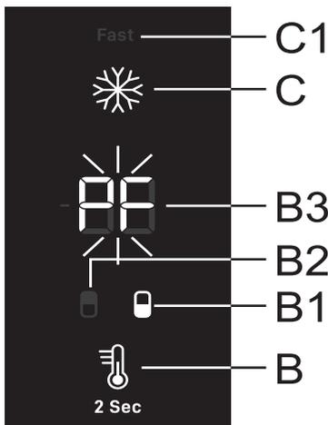
If the temperature in the appliance reached the alarm level during the power outage, then the high temperature alarm will be activated when power supply is restored. Acoustic alarm will be sounded, and **PF** will flash on the display unit **B3**.
