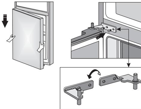
15. Correctly position the top door, run the connector (A) through the hole in the top hinge (3) and use the screws (2) to attach it. Hold the top door in place while positioning them. Reconnect the connector (A).
