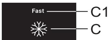
**Switching off:** If the refrigerator compartment is active (**B2** is lit up), then first press the **C** key to switch to the freezer compartment (**B1** will be lit up), and then press the **C** key to deactivate the function.
