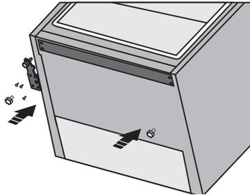
14. Place the bottom door onto the bottom hinge and hold them in place. Rotate the middle hinge by 180°. Place the washer in the correct position and adjust the position of the middle hinge so that you can install and fix the bottom door.
