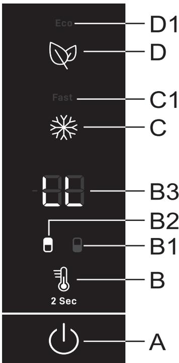
**Switching on:** To activate the child lock, press the **A** and **D** keys and hold them for two seconds. **LL** will briefly appear on the **B3** display unit.
