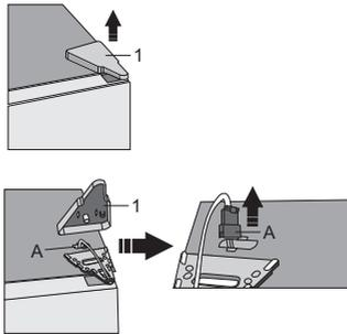
3. Undo the screws (2) and remove the hinge (3). Run the connector (A) through the hole in the hinge. Hold the door while doing this to prevent it from falling.
