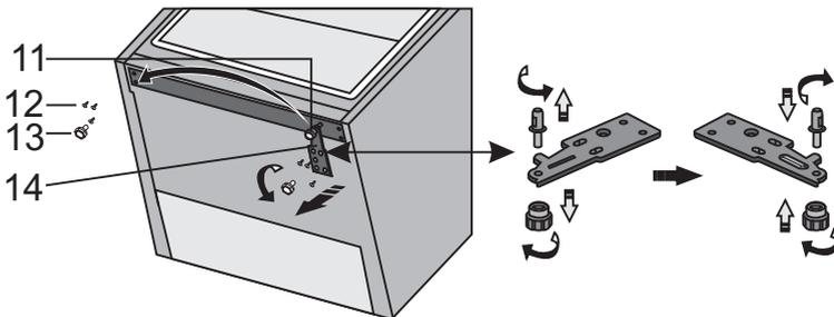
13. Use the screws to attach the foot from step 11 and the bottom hinge from step 12 to the opposite side.
