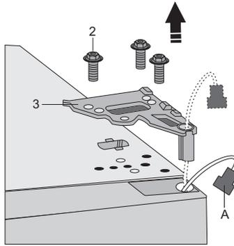
4. Remove the top door from the middle hinge by carefully lifting it straight up. Lay the door onto a smooth surface.
