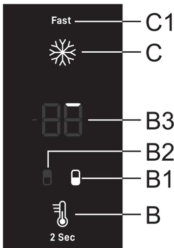
**To activate** the intensive freezing function, press the **C** key. You will hear a beep, indicators **B1** and **C1** will light up.
