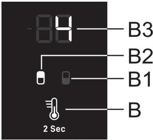
Temperature in the **refrigerator compartment** can be set when the **B2** symbol is lit. Set the temperature by briefly pressing the **B** key.
