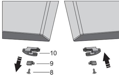
10. Remove the middle hinge cap and replace it on the opposite side.
