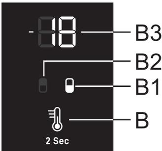
Temperature in the **freezer compartment** can be set when the **B1** symbol is lit. Set the temperature by briefly pressing the **B** key.
