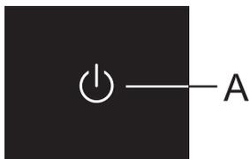
When you connect the appliance to the power mains for the first time, the appliance will be in standby mode (switched off, but powered).
