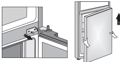
9. Lay the bottom door onto a smooth surface. Undo the screw (8) and remove the door retainer (10) and the door stop (9). Then, use a screw (8) to attach the door retainer supplied in the bag, and the door stop (9). Keep the door retainer (10) in case you need it later.
