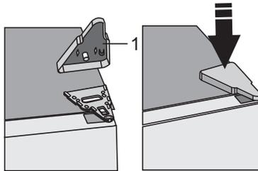
17. Open the top door and replace the door rack; then, close the door.
