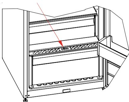
When the humidity controller in the closed position, it allows fresh fruit and vegetables to be stored longer.
