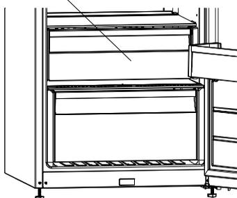
Keeping food in the Chiller compartment instead of the freezer or refrigerator compartment allows food retain freshness and flavour longer, while preserving its fresh appearance. When chiller tray becomes dirty, remove it and wash it with water.
