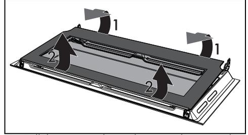
3. Pull the intermediate glass unit downwards from the door and then lift it upwards following the movement indicated by the arrows 2.
