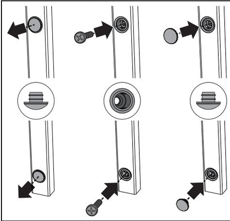
1. Remove the bushing covers on the front of the appliance.
