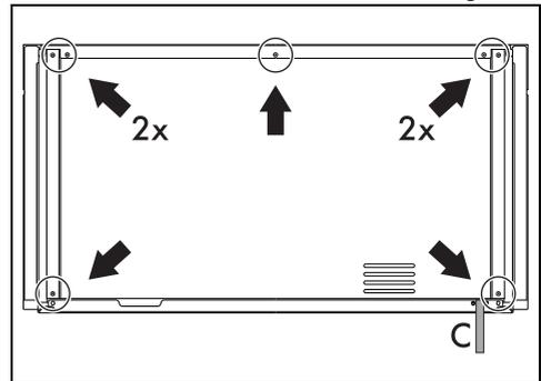
2. Lift the rear casing slightly and remove it to gain access to the terminal board.
