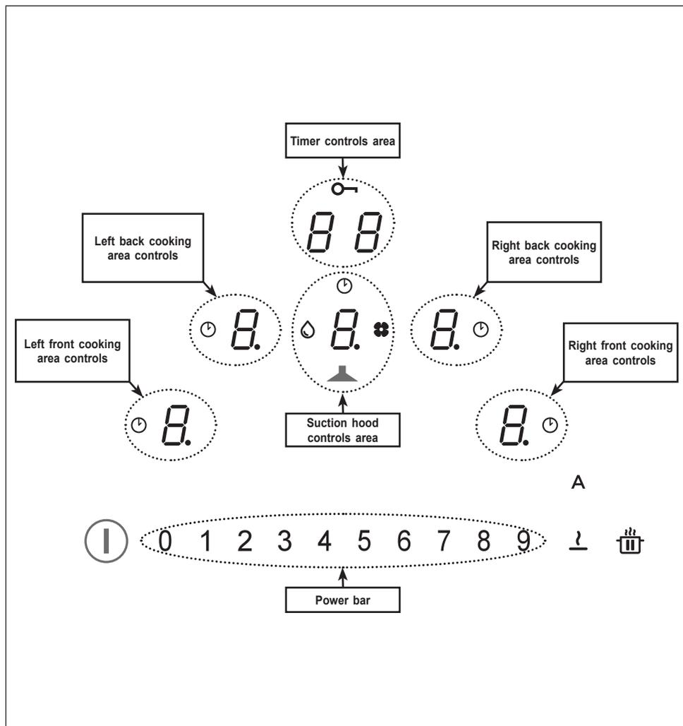
The controls for the cooking areas, suction hood and timer can be activated by pressing on the reference Digit 8. The Digit lights up more intensely to confirm the operation.
