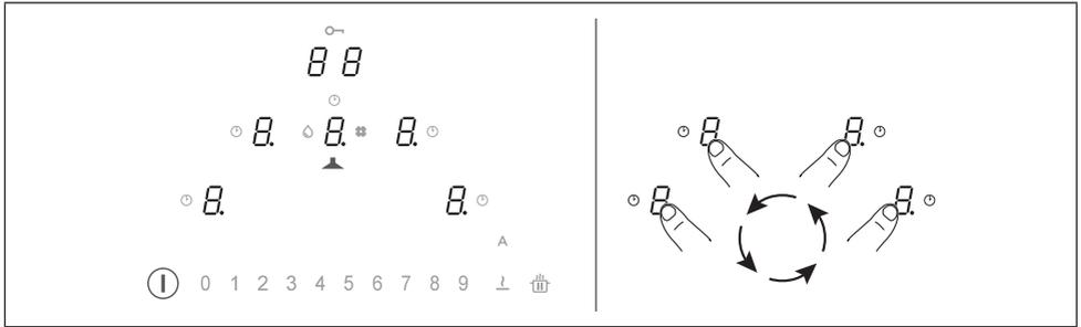
When first connecting to the domestic power supply, the installer must set the power of the hob cooking areas based on the actual abilities and capacity of the power supply itself.
