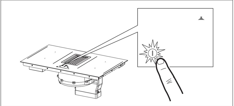
Press and hold the On/Off button
