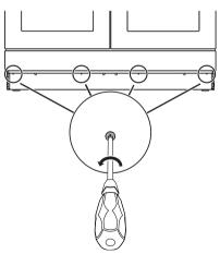
2. Align the front plinth with the corresponding holes on the appliance.
