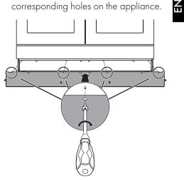
3. Fasten the front plinth using the screws that were previously removed.
