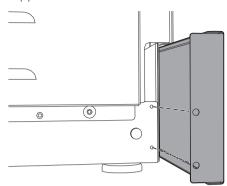
4. Fasten the side plinth using a screw.
