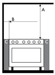
**A** 600 mm (Overhead) measured from the highest part of the highest burner and 750 mm for an exhaust fan.
