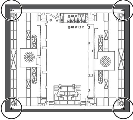
2. Remove the 4 screws from the corners of the appliance (1), position the supplied clips (2) and fasten them in place with the 4 previously removed screws and the 4 supplied screws (3).
