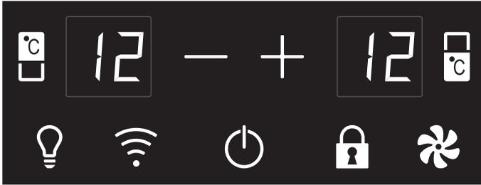
The control panel allows the user to interact with the appliance. Touch the keys with symbols to access the available functions.
