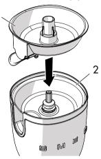
2. Insert the filter (3) in the juice collector and then place the reamer (4) on top of the filter.
