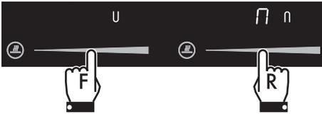
The displays of the cooking zones will turn on: the display shows the "master" **U** symbol while the right-hand display shows **n** followed by the "slave" **n** symbol.
