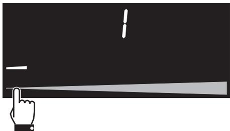
The display of the cooking zone used will turn on: the power value indicated is **1**.
