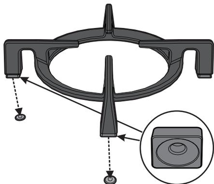
Make sure that the grids are simply centred on their respective burners, without forcing the burners to be raised or tilted. If this is the case, repeat the positioning procedure.
