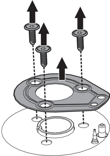
5. Unscrew the 6 screws that hold the glass hob top to the casing (see the figures below for their location).
