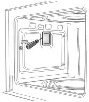
Slide out and remove the light bulb.
